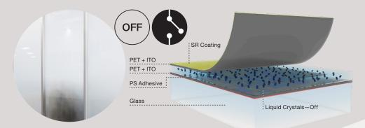
In the absence of an electrical current, the liquid crystal particles disperse randomly, scattering light which results in a translucent appearance.
