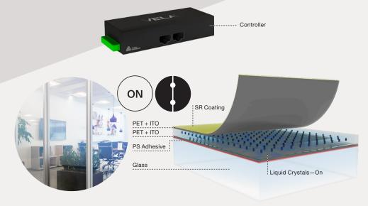
Activating the Vela<sup>™</sup> film introduces electricity to the film which causes the liquid crystal particles to orient in a manner that permits light to traverse the film and results in a transparent state.
